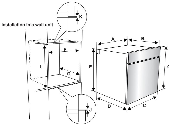
After making the electrical connections, insert the oven into the cabinet by pushing it forward. Open the oven door and insert 2 screws in the holes located on the oven frame. While the product frame touches the wooden surface of the cabinet, tighten the screws.
